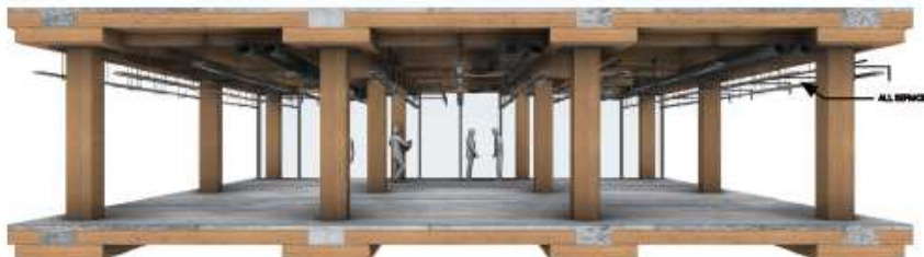
CLT / Concrete Composite System Full CLT structure acts as formwork for concrete screed and beams
